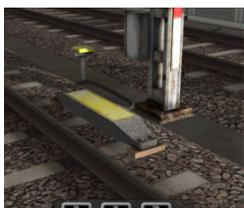
PZB is implemented by means of three kinds of magnets that are placed on the track; these are described as 500Hz, 1000Hz and 2000Hz. These magnets are only powered if their associated signal is set at a non-clear aspect, if the aspect is clear ('green / green') then the magnets have no effect on the train.
