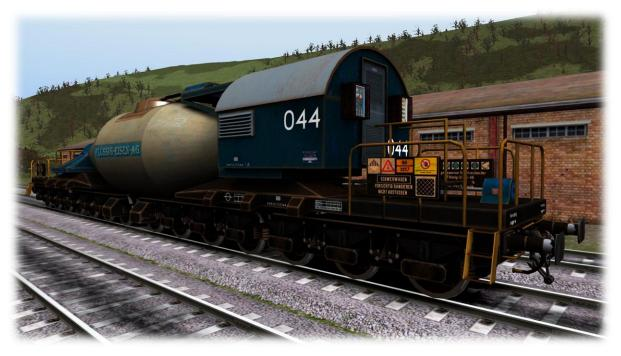
These are special wagons with which molten iron is transported from the furnace to the foundry. Through their dual fireclay insulating the iron can be kept liquid at a temperature of about 1,400 degrees Celsius for up to 30 hours. Since these wagons are exposed to aggressive substances at a high temperature, they grow very fast and are covered with a layer of rust after a short time.
