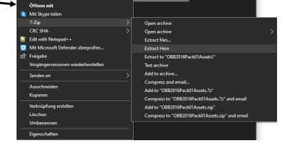
Unpacking is urgently required, otherwise the installer (Step 6) will not be able to find and copy the required model and script files, which means that the vehicle cannot be installed.
