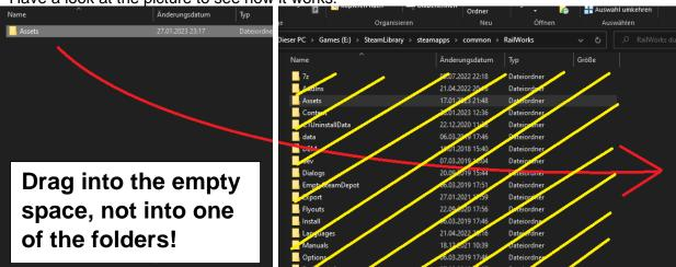
If Windows asks you whether you want to replace files, then have them replaced, otherwise the Desiro HC will not work. The following will be replaced: The FIS file and the old files of the first version of the Desiro HC (if it was installed).
