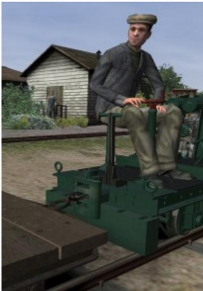
The coupling for Lister Rail - Trucks reflected the rest of the loco. In the early days it was a simple bent metal bar but most pictures from the 1930's onwards show a similar design of coupling which acts as both buffer and receiver for a chain.
